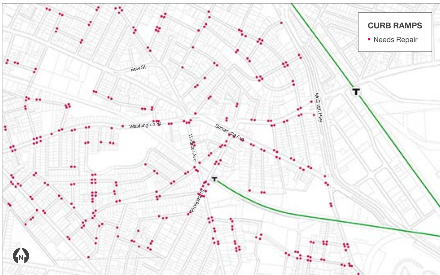
BELOW: Using the 2013 Pedestrian Accessibility Study, an input in the Neighborhood Streets Reconstruction Program, existing sidewalk ramps were surveyed and catalogued. Ramps needing repair to comply with MAAB standards were identified.
