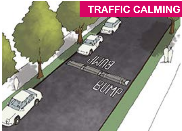
ABOVE: Speed humps are rounded, raised portions of the roadway 10-14' long and 3-4" high. They are distinct from the other "speed bumps" found in many parking lots, and often tapered at the curb to allow for unimpeded drainage.
