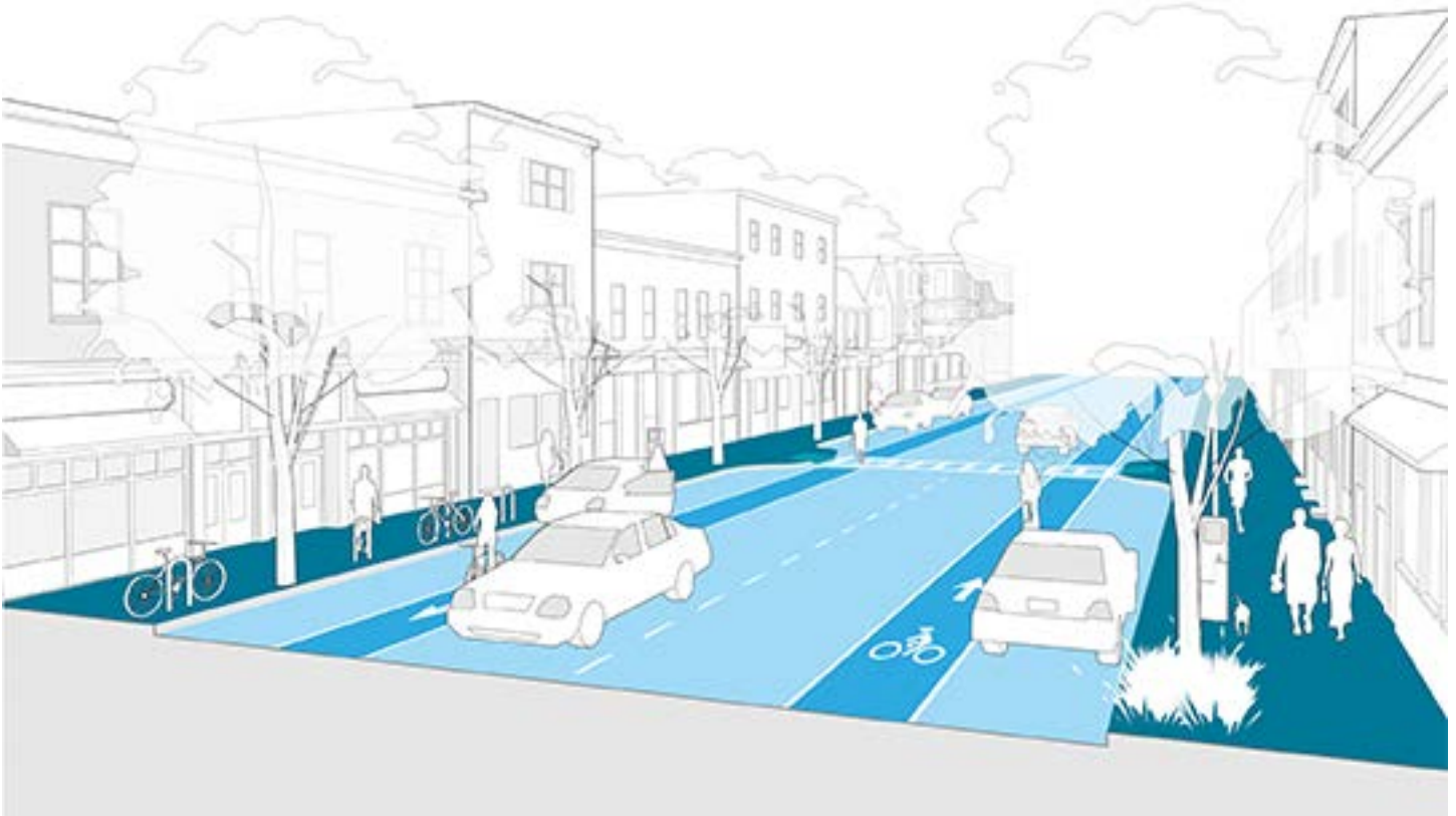
ABOVE: A graphic from the Boston Complete Streets Guidelines showing wide sidewalks, parking, a bike lane, and crosswalk including a bump out.
