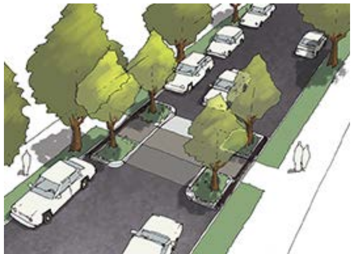
ABOVE: Pinch points are curb extensions aligned at mid block locations to narrow a street down to one travel lane. Pinch points may include a crosswalk and/or landscaping in a curb extension.
