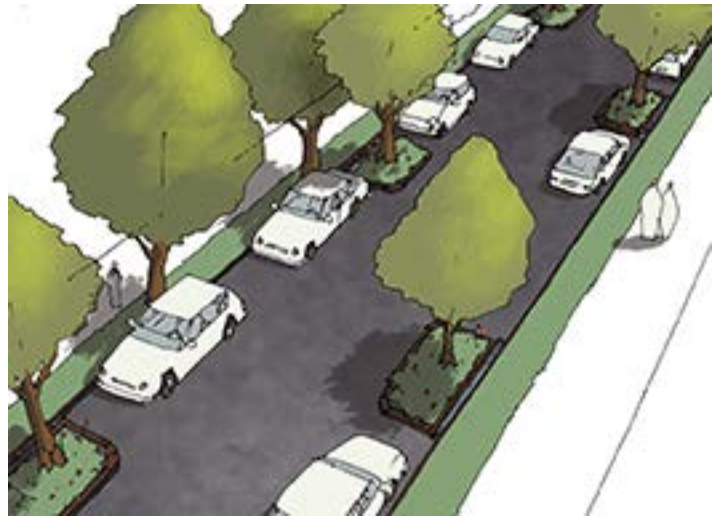
ABOVE: Parking lane planters decrease traffic speed in two ways by physical narrowing the roadway similar to on-street parking and creating "visual friction" in the peripheral vision of drivers.
