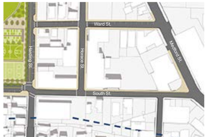
ABOVE: South Street in the existing segment from Medford Street to Harding Street is wide enough to change to a two-way street with no on-street parking. This can be done with little interruption since the segment isn't signalized.
