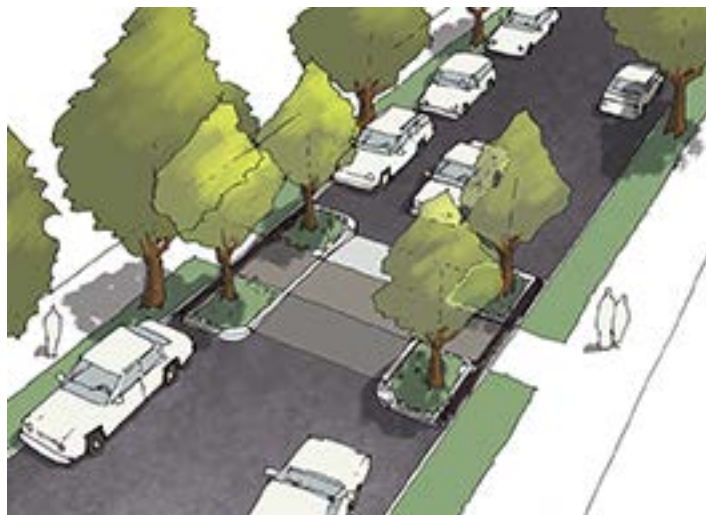
ABOVE: Pinch points are curb extensions aligned at mid block locations to narrow a street down to one travel lane. Pinch points may include a crosswalk and/or landscaping in a curb extension.
