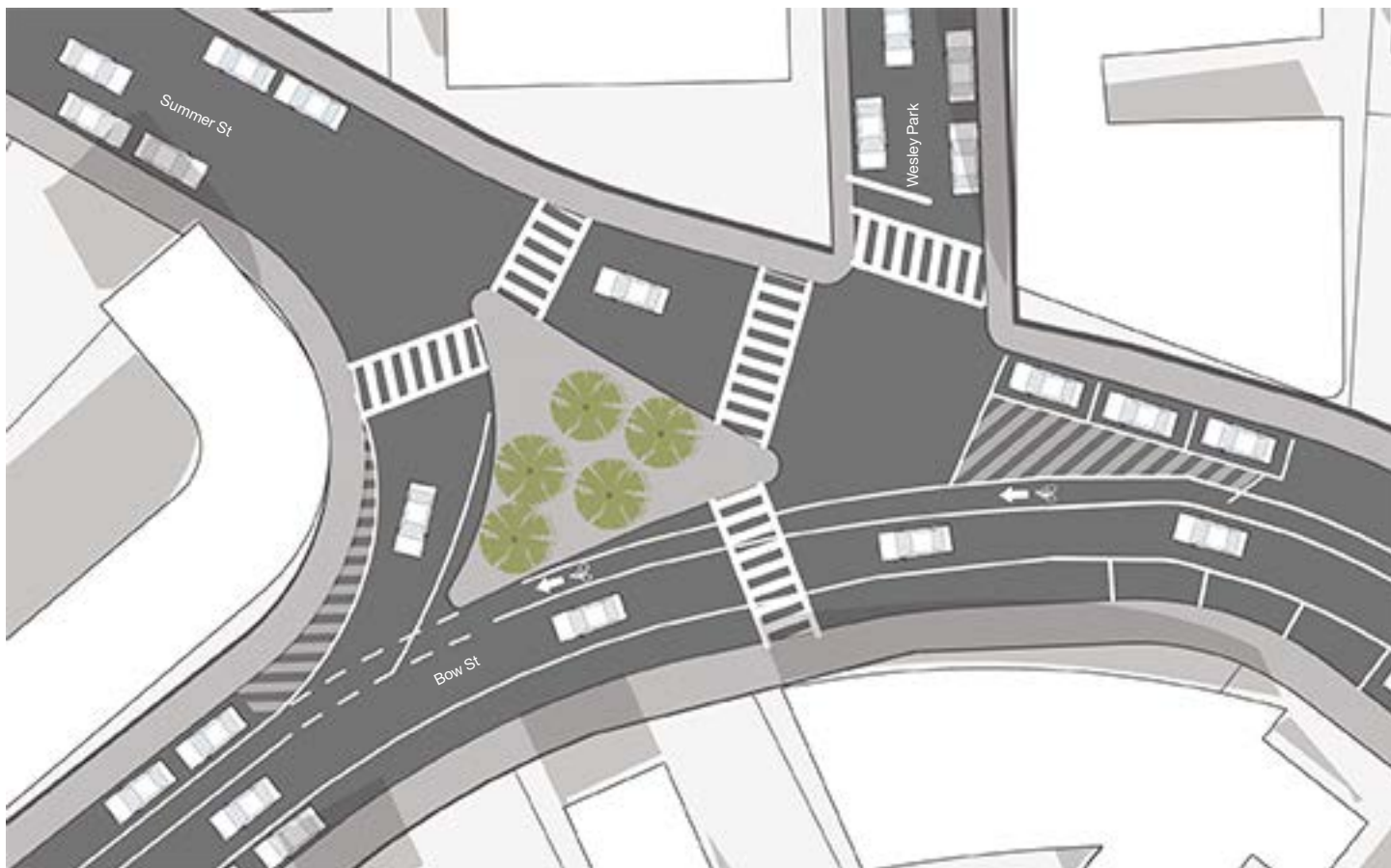
ABOVE: The intersection of Bow and Summer Street is confusing. Cars entering Summer Street can do so quickly and in a straight shot but have to yield to cyclists. Cars can enter Bow Street from Summer Street without stopping. The majority of pedestrian crossings are signaled because of the roadway.
