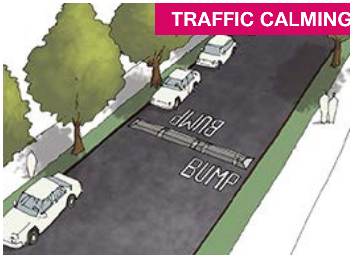
ABOVE: Speed humps are rounded, raised portions of the roadway 10-14' long and 3-4" high. They are distinct from the other "speed bumps" found in many parking lots, and often tapered at the curb to allow for unimpeded drainage.
