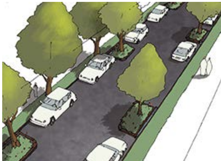
ABOVE: Parking lane planters decrease traffic speed in two ways by physical narrowing the roadway similar to on-street parking and creating "visual friction" in the peripheral vision of drivers.
