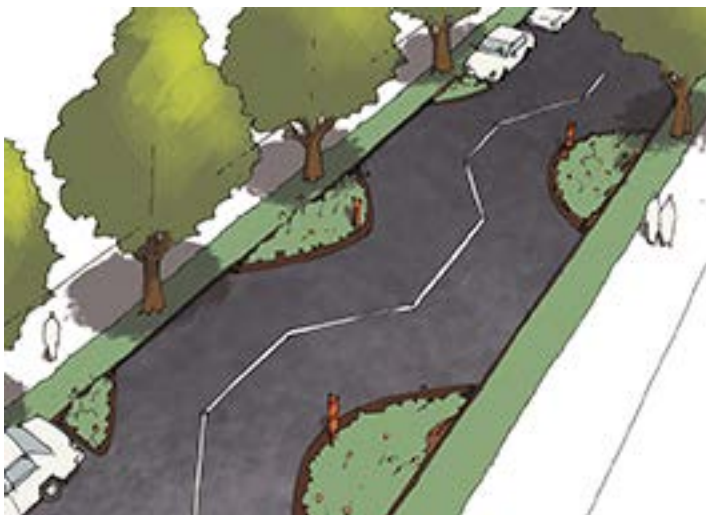
ABOVE: Chicanes are staggered curb extensions installed on alternating sides of the street that reduce vehicular speed by requiring drivers to maneuver through the extensions. The calming effect depends on how far the chicane extends into the roadway and can be replicated by alternating on-street parking on one side of the street and the other.
